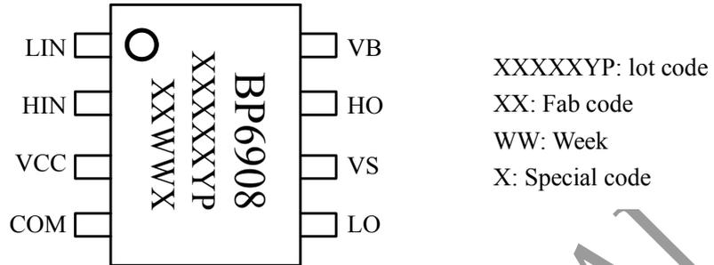
Figure 2. Pin configuration
